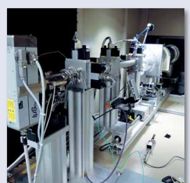
\mu S and SCATEX upgrade on a customized SAXS setup in Hamburg
