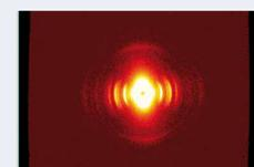
Detector image of a SAXS experiment: sample rat tail tendon
