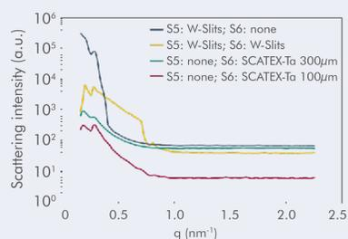
Scattering intensity vs. q-plot deduced from an integration along a full circle and normalized to the number of summed up pixel. Various apertures were tested at position S5 (beam definition) and S6 (scatter guard) (top).
