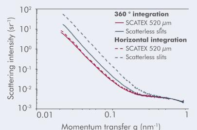
Scattering intensity vs. q-plot deduced from the integration in horizontal direction with an opening angle of 5° and from an integration along a full circle. The data is normalized to the photon flux downstream of the test aperture and to the solid angle.
