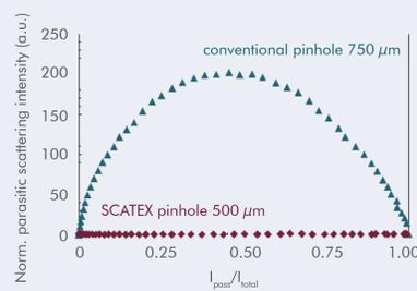
Measurement results of a SCATEX Ge and a conventional Pt/Ir pinhole. The apertures are driven stepwise into the X-ray beam while simultaneously measuring the parasitic aperture scattering around the beam stop. The parasitic scattering intensity is corrected for the dark current of the detector and for air scattering. The signal is normalized to a standard glassy carbon intensity in order to allow a comparison.
