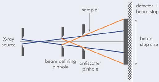
A SAXS setup with a typical 3-pinhole collimation system. This illustration clearly shows that even with an antiscatter pinhole the beam stop needs a large diameter due to the parasitic scattering. With SCATEX pinholes the antiscatter pinhole becomes dispensable and the beam stop only needs to have the size of the primary beam. This enables a higher resolution and photon flux.
