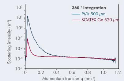
Scattering intensity deduced from the detector images and corrected for the different measurement times and normalized to the photon flux upstream of the tested aperture.
