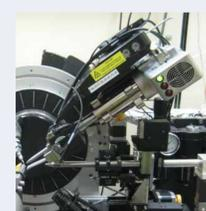
Mo- $1\mu\text{S}$  as second source at small-molecule beamline 11.3.1 at ALS
