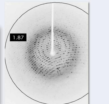
Data statistics and typical diffraction pattern of a protein complex, recorded with a D8 VENTURE 2<sup>nd</sup> Gen. and the METALJET X-ray source using a Ga rich alloy. The good data quality allowed for a structure solution by molecular replacement.
