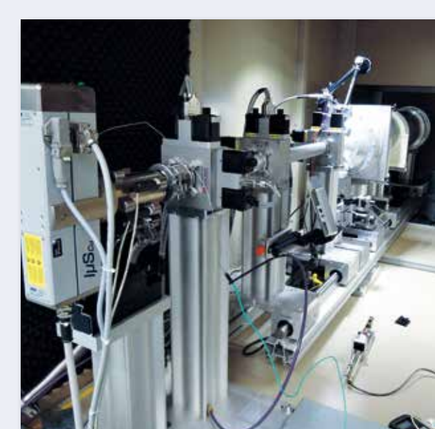
\mu S and SCATEX upgrade on a customized SAXS setup in Hamburg
