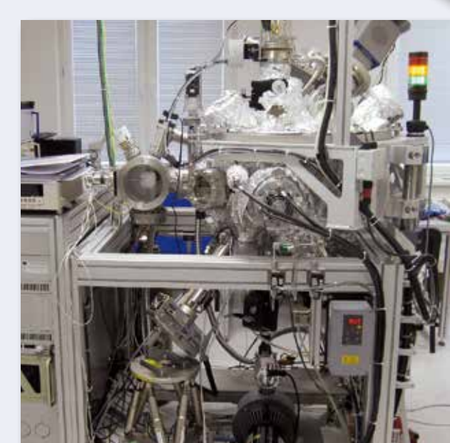
Adaptation to UHV deposition chamber for in-situ GISAXS studies in Bratislava, Slovakia
