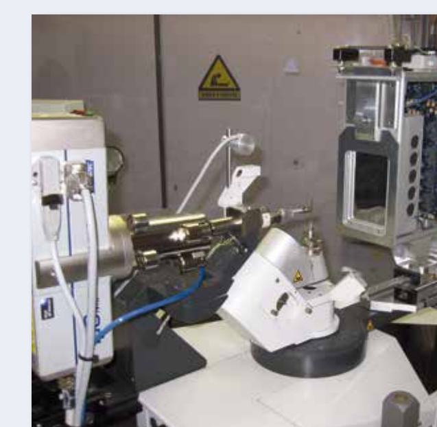
SCD setup for time resolved experiments w/ XPAD detector in Nancy, France
