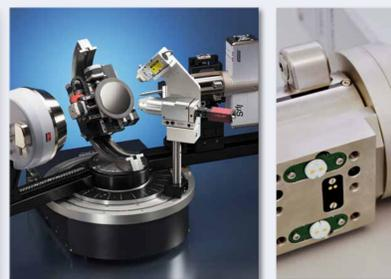
D8 Advance: XRD $^2$  system with  $I\mu S^{\text{High Brilliance}}$  (left). Integrated memory chips store information provided by the manufacturer and during use (right).
