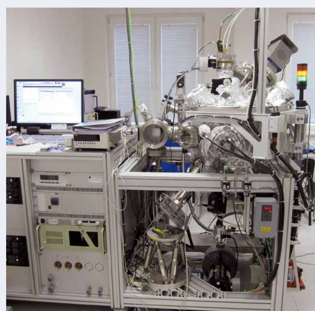
Hexapod adaptation to UHV deposition chamber for in-situ studies in Bratislava, Slovakia
